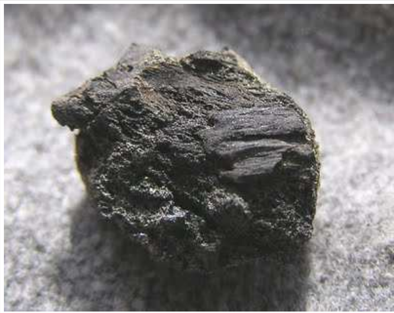
1 cm nodule of charcoal, still showing original wood grain, surrounded by a rind of bisqued clay.
